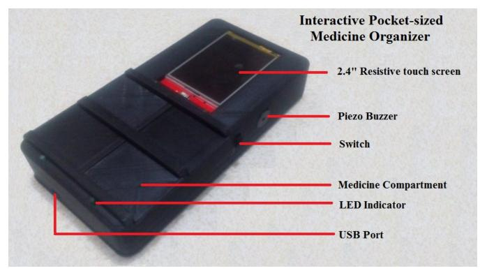
Fig. 1. Working Prototype of the Pocket-sized Electronic Pillbox Device
