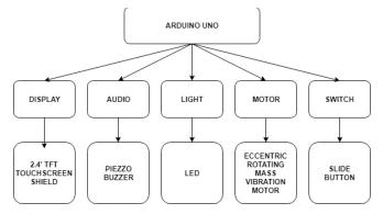
Fig. 3. Decomposition of Hardware Modules
