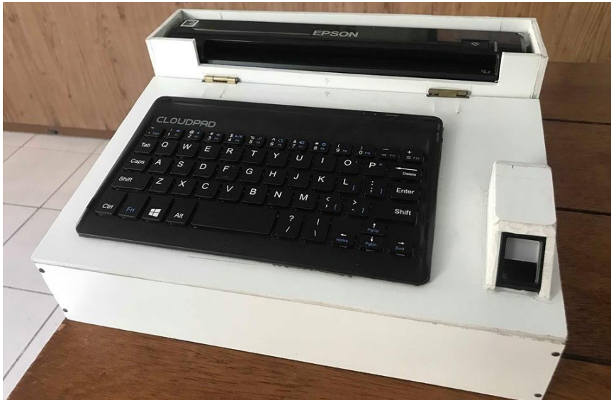
Figure 5: The VISIMP Portable Communications Device for Visually Impaired Individuals
